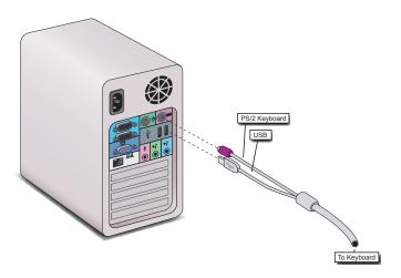
Figure 1 Cable Connections to the PC
