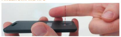
» Line up the first crease of your finger with the center of the sensor.
