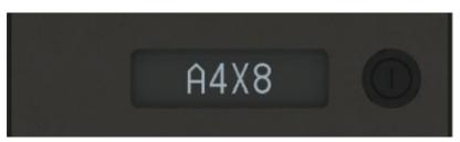
» If enrollment is successful then you will be shown a four-character code on the B-Unit 3 display. If you were not able to enroll, you can try again by turning the B-Unit 3 back on and repeating the enrollment procedure from that step.
