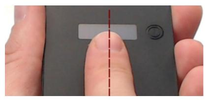
» Make sure your finger is straight along the center of the B-Unit 3 and that you swipe in a straight line downward over the sensor.
